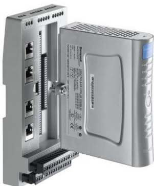
Figure 5. RTU Processor ease of removal from IOTA
